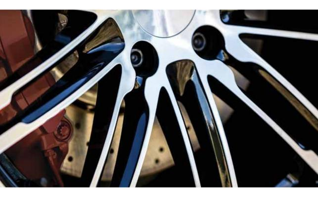
Jotun Primax Diamond is tailor-made for machined wheels, offering superior corrosion and stone chip protection. It also has the perfect surface and consistent quality throughout.
